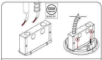
For Optional Junction Box Housing install, knock out desired box entry. Connect fitting and supply cable Mount to Diecast Plaster Plate with supplied srews.
