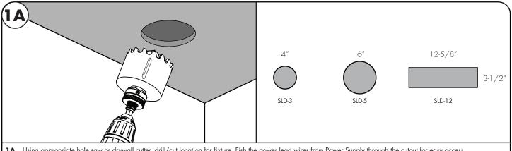
1A Using appropriate hole saw or drywall cutter, drill/cut location for fixture. Fish the power lead wires from Power Supply through the cutout for easy access.
