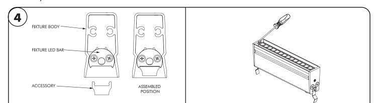
Optional lens accessories can be simply snapped into the fixture LED bar to secure.
