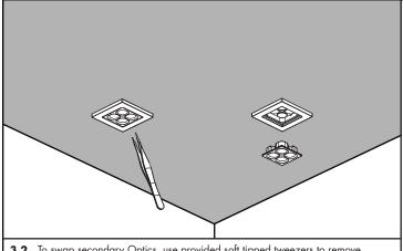
**3.2** To swap secondary Optics, use provided soft tipped tweezers to remove existing magnetically attached louver and install desired version.
