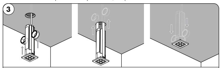
3.1 Unroll the constant force springs from both sides of the fixture. Then place them inside the round cut out one side at a time. Slowly allow the fixture to slide into hole as the constant force spring pull up the fixture
