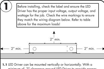
minimum of 2" clearance around LED Driver to provide proper air circulation.
