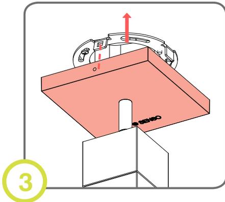
3 Line up canopy with crossbar's screw holes, slide onto ceiling.
