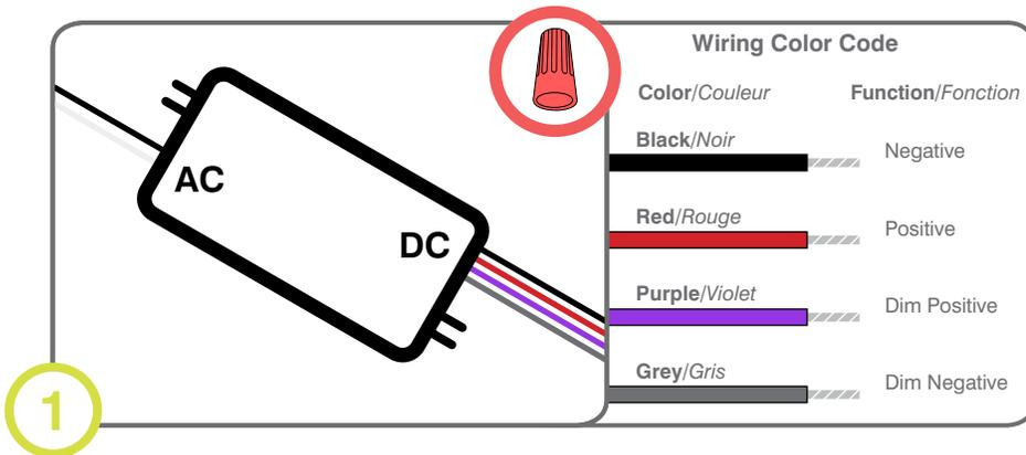
1 Make AC connections to ceiling and place driver in junction box. Orange wire is not used and should be capped.
