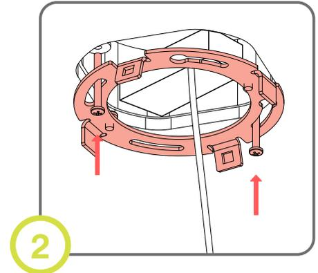
2 Screw bracket onto junction box and make DC connections to fixture.
